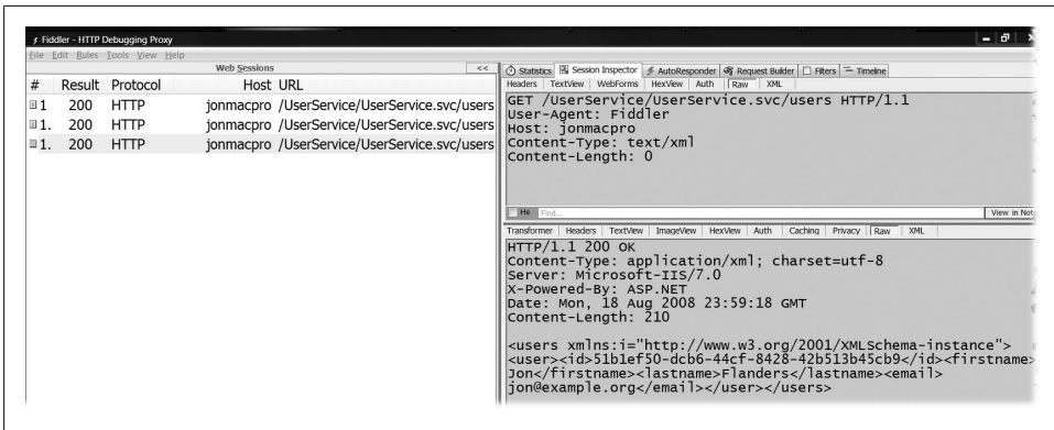
Figure 4-6. Fiddler Session Inspector view of a GET request showing a newly added user resource
